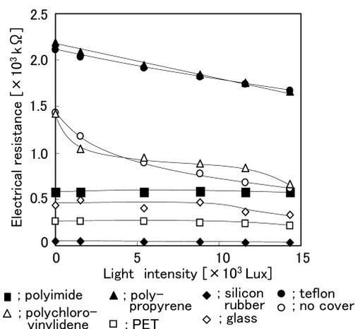
Fig. 6 Relationship between the electrical resistance of microsensors packaged with various materials and the intensity of light irradiation onto the sensors
