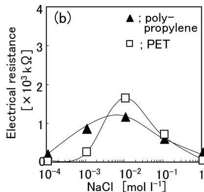
Fig. 3 Relationship between the electrical resistance of the microsensor and the concentration of the NaCl solution (b)
