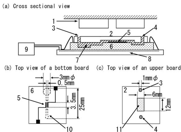
Fig. 1 (a) Schematic diagram of the measurement system for determining optical and concentration sensitivity of a microsensor. (b) Top view of the bottom board. (c) Top view of the upper transparent board
