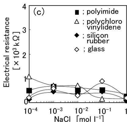
Fig. 4 Relationship between the electrical resistance of the microsensor and NaCl concentration (c)
