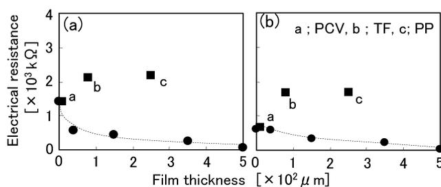
Fig. 7 Relationship between the electrical resistance of the microsensor and the film thickness of the upper board
