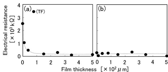
Fig. 5 Relationship between the electrical resistance of the microsensor and the film thickness of the upper board
