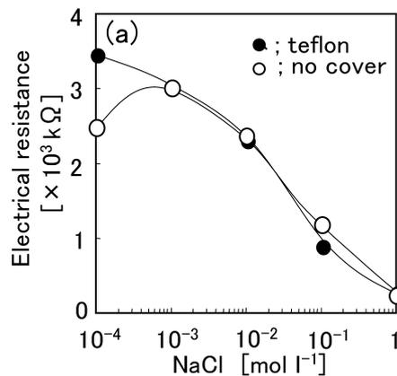
Fig. 2 Relationship between the electrical resistance of the microsensor and the concentration of the NaCl solution (a)
