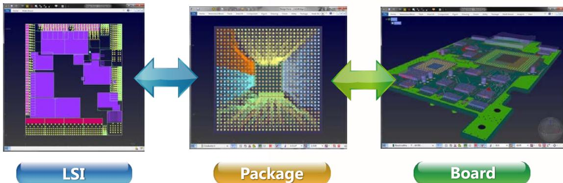
A multi-technology / multi-object environment which shows systems and modules having a complex hierarchical structure, similar to LSI/PKG/PCB, as a single unit is a powerful tool for considering total optimization trade-offs.
